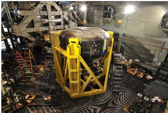
Image 4. NASA's Composite Crew Module (CCM) in the test rig (upside down) at NASA's Engineering and Safety Center (NEC) at Langley Research Center. The CCM project is being carried out to study materials tradeoffs between metals and composites in large space structures. Photo courtesy of NASA [EDITORS NOTE: A similar photo is also available in a vertical format] # # #
