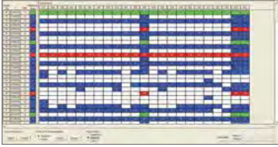
Figure 2: The data in HyperSizer can be formatted in Excel spreadsheets and color codes matched to either FiberSIM or CATIA for direct export. In this HyperSizer screen shot, with the FiberSIM box checked (lower left), the color code represents the following: blue signifies 0-degree fiber orientation; green denotes +45 degree; and red is -45 degree. The software can also be set to match CATIA's standard color codes. (Note that this static screen shot displays only a portion of the laminate thickness that can be seen when actually using the software.)
