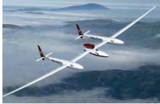
Figure 1: The aerodynamic similarities between long, thin aircraft wings (such as those on Steve Fossett's Global Flyer, top) and modern wind turbine blades can be used to guide design blade decisions. Composites manufacturing lessons learned in aerospace can also be applied to wind blades (left).
