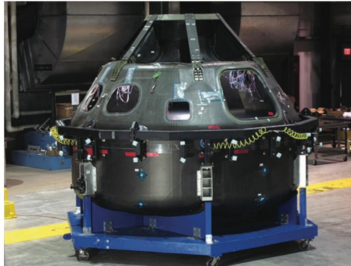
The design and construction of the NASA Composite Crew Module was optimized with the help of HyperSizer structural sizing and design analysis software. The module is pictured here with sensors attached in preparation for pressure testing.
