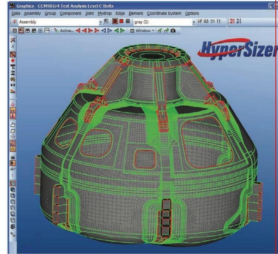
This finite element model of the CCM displayed in HyperSizer shows the composite ply drops identified in green.
