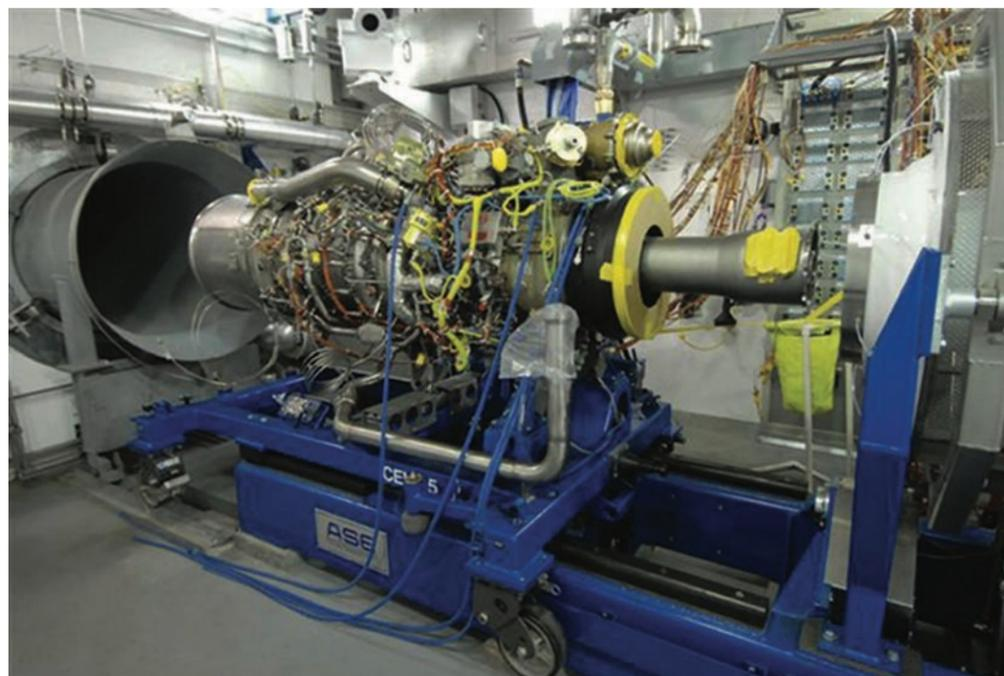
Factory testing of the GE38 at GE's test cell in Lynn, MA, is expected to run through 2011 in concurrence with a full military qualification test program.
