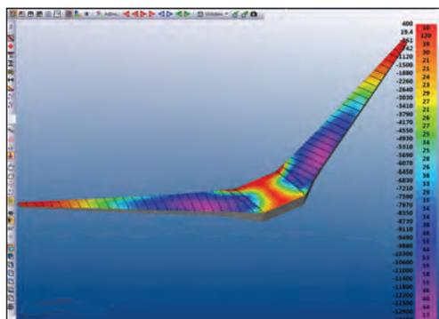
**Fig. 2** – A HyperSizer screen shot shows a FEA-computed axial running load for airframe stiffened panel skins, where purple indicates peak compressive force. HyperSizer iterates in an automated loop with FEA software to calculate the most lightweight and robust design options.
