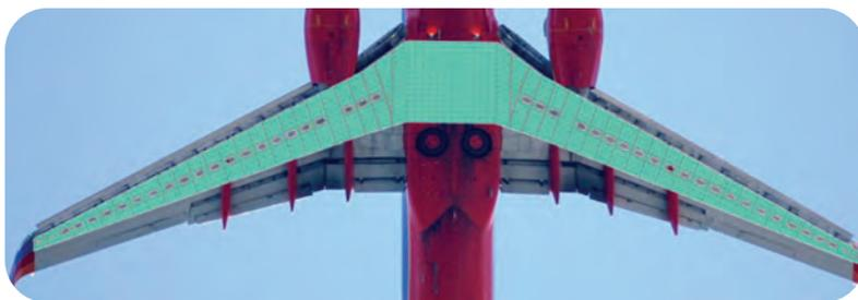
**Fig. 1** – Finite element model highlights load-carrying wing box structure (the section of the fuselage between wing roots) for a commercial aircraft. HyperSizer structural sizing and composite analysis software complements FEA in optimizing wing box and other airframe structure designs by reducing weight while maintaining structural strength and improving manufacturability.
