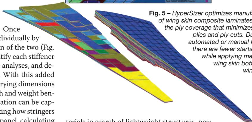
**Fig. 5** – HyperSizer optimizes manufacturability of wing skin composite laminates by finding the ply coverage that minimizes individual plies and ply cuts. During either automated or manual fabrication, there are fewer starts and stops while applying material. Left, wing skin bottom. Right, wing skin top.
