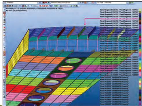
**Fig. 4** – A discrete model of a stiffened airframe panel design. Individual panel segments (varying colors) are automatically identified by HyperSizer and used for analysis.
