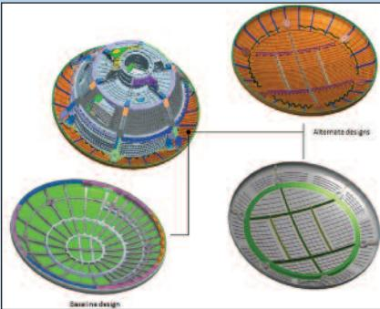
HyperSizer evaluated different structural concepts for the heat shield carrier structure. The baseline composite skin with Titanium I stringers (left, bottom) was evaluated against alternate metallic grid stiffened designs (right, top and bottom).
