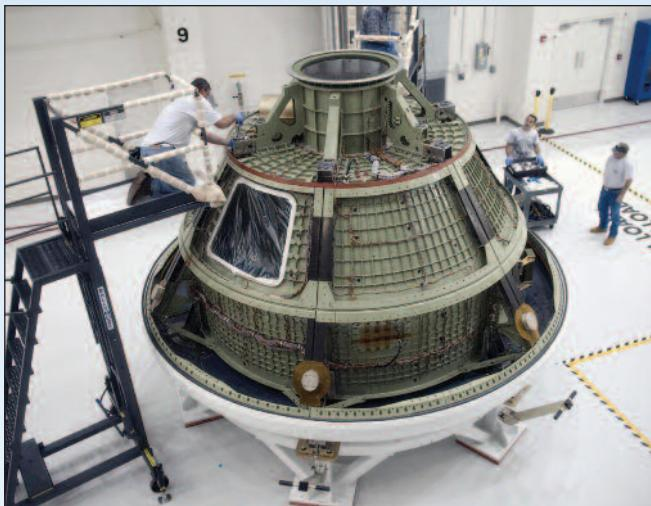
The Orion ground test vehicle at NASA's Kennedy Space Center. The circular heat shield is visible at the very base of the vehicle. (NASA)
