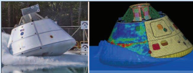
(Left) The Orion Multi-Purpose Crew Vehicle splashdown test, and (right) software simulation of loads on the vehicle during the highly dynamic event.
