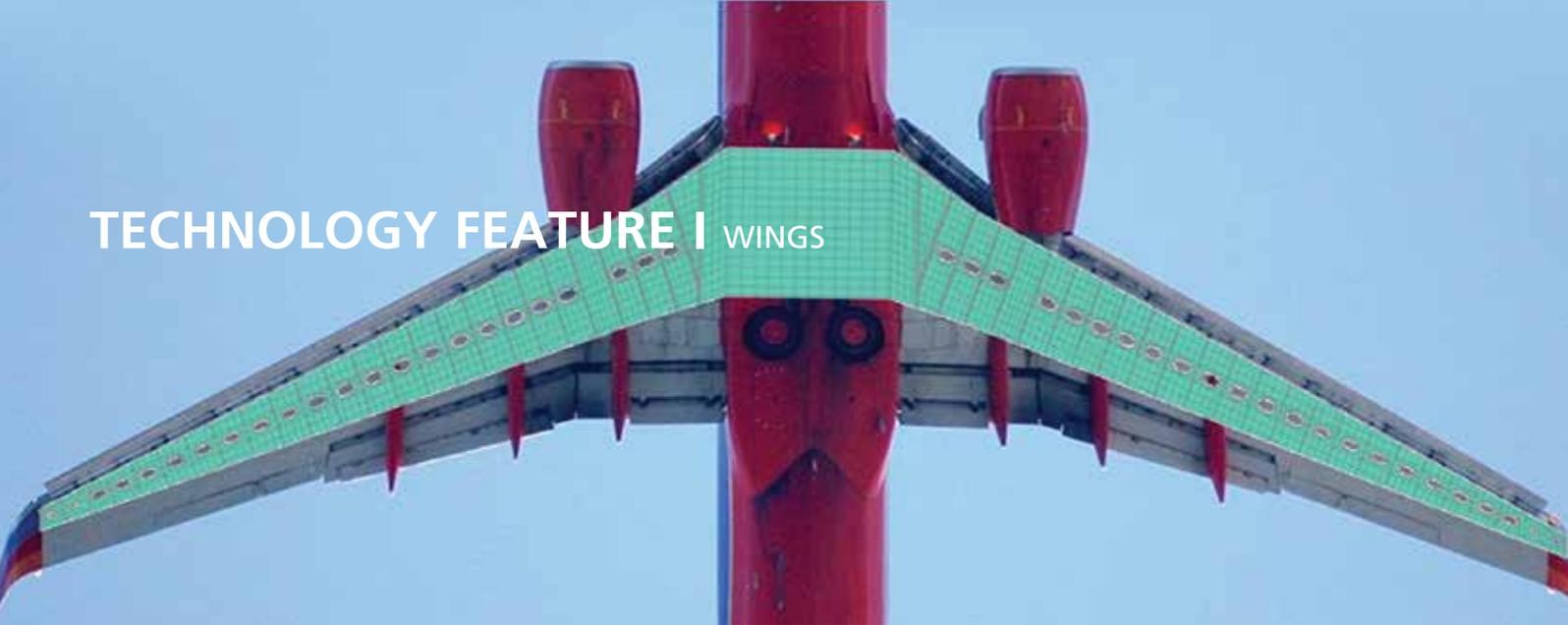
This finite element model highlights the load carrying wing box structure (the section of the fuselage between the wing roots) for a commercial aircraft
