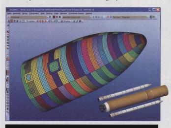
NASA engineers recently analyzed the composite shroud that's part of its Ares V space launch vehicle. The simulation is pictured. The engineers paired FEA and composite-analysis software to find the best dimensions and composite materials for the shroud.
